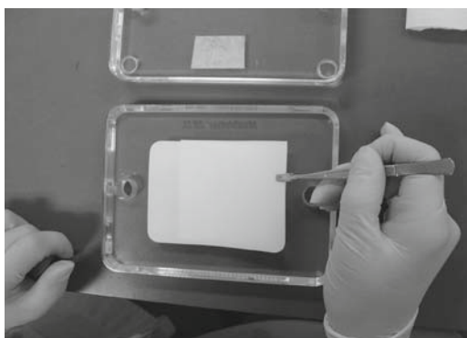
Fig. 5. A plastic cushion is placed onto the NC.
