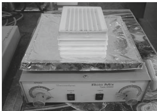
Fig. 17. Incubation for 90 min at RT on a shaker.
