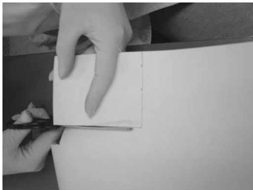
Fig. 1. Cut a rectangle of NC sheet 7.5 \times 10 cm.
