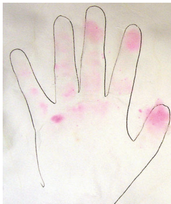
Fig. 4. Hand imprint, developed by the dimethylglyoxime (DMG) test, indicating skin areas contaminated by nickel after 30 min of manipulating nickel-releasing tools (Fig. 3). The imprint was taken on blotting paper moistened with nitric acid (1%), and the contour of the hand was marked. The imprint was developed with DMG solution and ammonia after drying. The pink colour on the paper indicates nickel transferred from the skin that had been contaminated by the tools.
