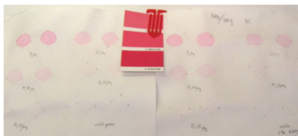
Fig. 2. Test of nickel concentration curve on blotting paper, to visualize the lowest concentrations on paper that can be detected by the dimethylglyoxime test. Thirty millilitres of the stock solution (100, 50, 25, 10, 5 and, 0 µg/ml) was added to the blotting paper, corresponding to 3, 1.5, 0.75, 0.3, 0.15 and 0 µg of nickel, distributed over 3 cm 2 each. No pink coloration is seen with 0 and 0.15 µg of nickel. Weak pink colour is visible at 0.3 µg, which is considered to easily be missed. Obvious pink colour is present at 0.75 up to 3.0 µg.
