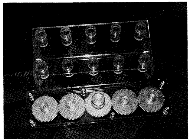
Fig. 1. Two parts of the new device. Front : circulating gears. Back : allergen extract tanks.
