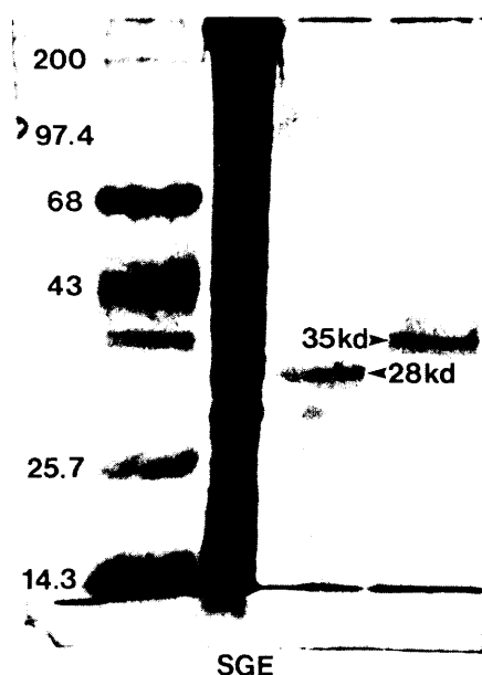
Fig. 4. Silver stain of SGE and electroeluted 28- and 35-kd allergens. Molecular weight standards \times 10^{-3} kd.
