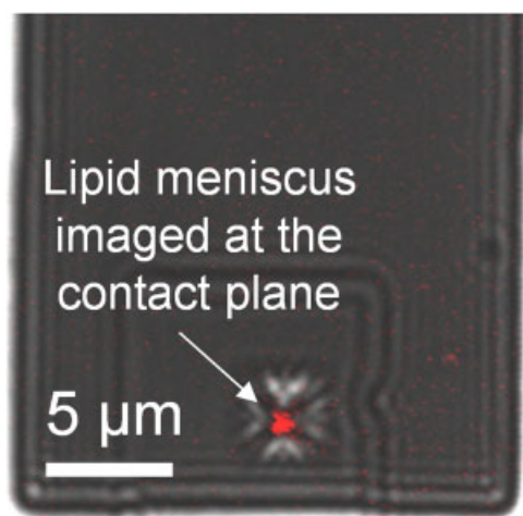
Fig 6. Confocal section (red) overlaid with a bright-field image (gray scale) taken after ~1 h under water. The meniscus is still visible at the contact point of the tip on the left as a red spot, although, at a diameter of less than 1 μm, it is significantly smaller than it was initially.
