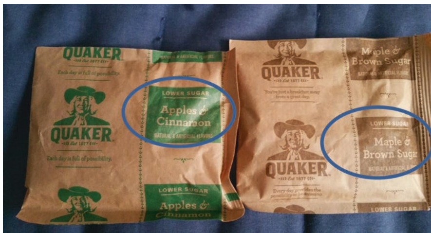
Fig. 6.6 An example of how a color difference or text difference can be used for detection by a vision system (Courtesy: PepsiCo, Inc.)
