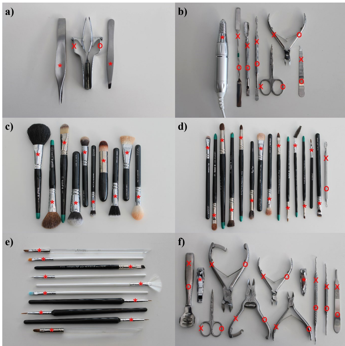
Figure 1: Tested instruments alongside with pre-determined testing sites. Nickel spot test testing sites are marked with an x, whereas cobalt spot test testing sites are marked with a circle (o). Asterisks (*) indicate testing sites where nickel and cobalt spot tests were performed on the corresponding opposite sides of the metal tool. a) tweezers (customary models as well as automatic tweezers, displayed in the middle), b) tools for conducting nail treatments (manicures), c) makeup brushes for application of liquid/cream products (concealer, foundation, liquid bronzer, liquid blush etc.) and powder products (setting powder, blusher, bronzer etc.), d) makeup brushes for application of eyeshadow (powder or liquid/cream) and/or eyebrow and eyelash products (mascara, eyebrow gel etc.) as well as a so-called blackhead remover (displayed on the right outer side), e) nail design/art brushes used for conducting nail treatments (mostly acrylic nails and gel nails), f) tools used for conducting pedicures
