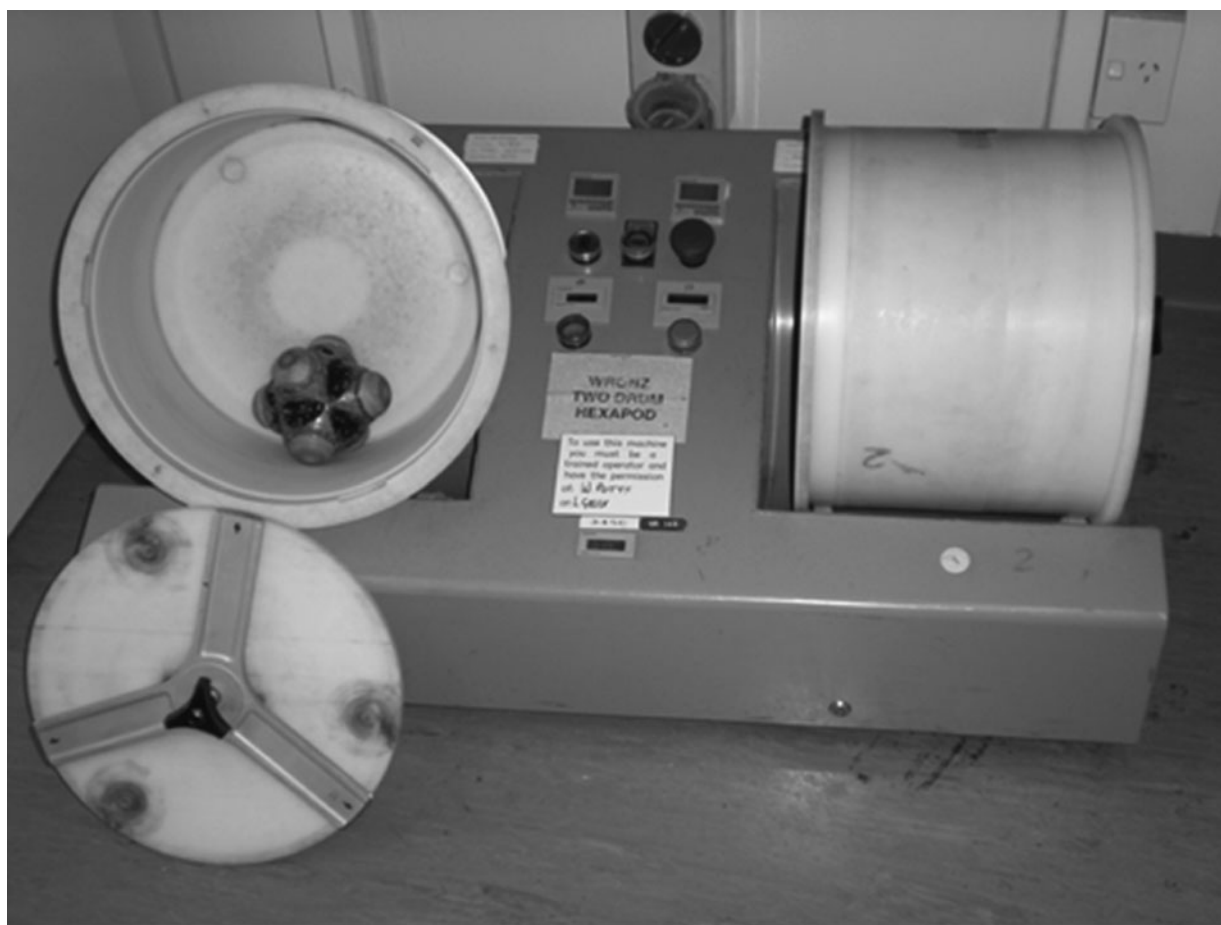
FIGURE 1. Hexapod-carpet wearing machine
