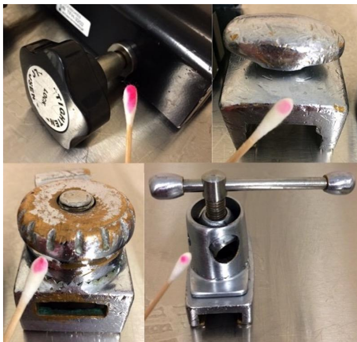
Figure 3. Photos of a variety of the operating table clamps that tested positive for nickel release.
