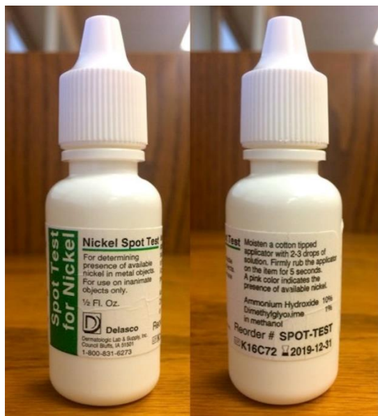
Figure 1. Photos of the nickel spot test used to test for nickel release. Delasco Dermatologic Lab & Supply, Inc. Spot Test For Nickel. Contains 1% dimethylglyoxime and 10% ammonium hydroxide.
