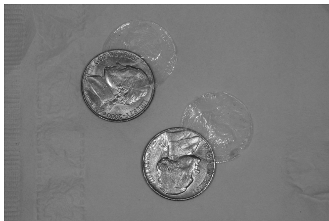
Figure 1. When nickels coated with three, four, or five coatings of Orly Nail Lacquer were soaked in saline for 2 days, the coatings peeled off of the nickels.
