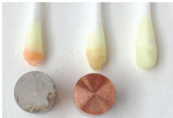
Fig. 1. Cobalt spot testing. From left to right: control (negative), copper, and cobalt. The reaction observed with copper is not considered to be a false-positive reaction, but does show a brown/rust-colour that is different from the negative control.
