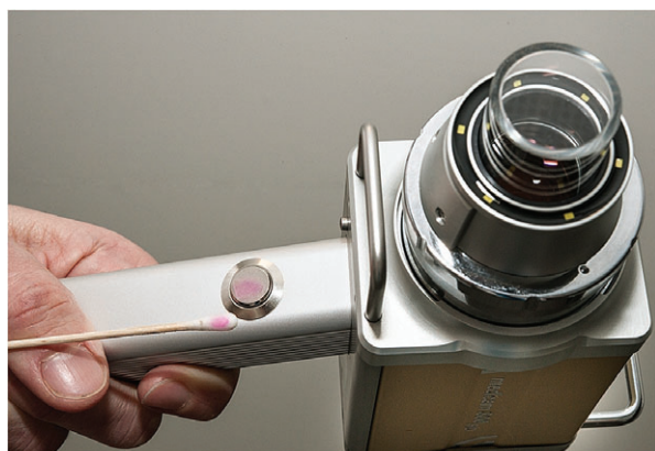
Fig. 1. Nickel release from the button of a Fotofinder ® dermoscope as indicated by positive dimethylglyoxime test reaction.
