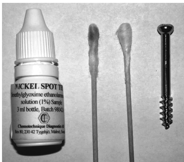
Figure 4. After surgical removal of the metal screw from the patient's elbow, a nickel spot test on the screw produced a pink color change on the cotton tip.
