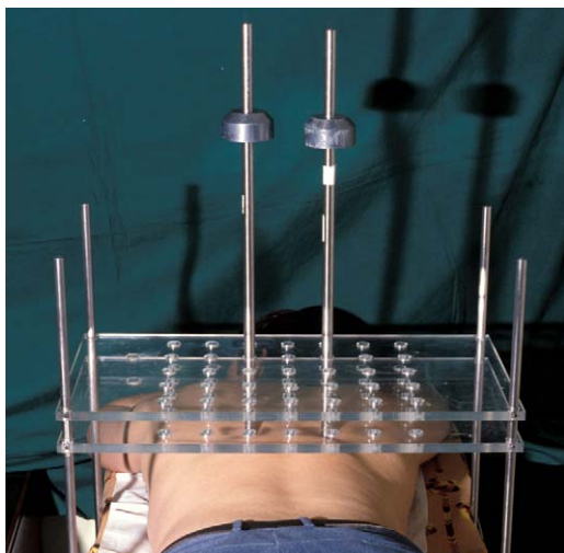
Fig. 2. Pressure instrument adapted from Illig and Kunick [20] with weighted rods resting on a patients' back.
