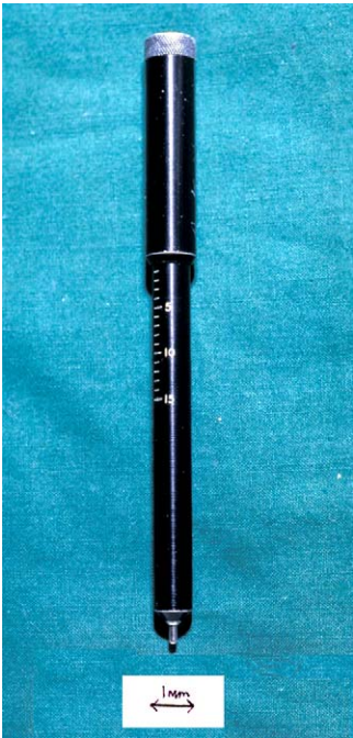
Fig. 4. A calibrated dermographometer. The setting of 10 on this dermographometer corresponds to a pressure of application of 9.75 \times 10^5 Pascals. The tip is pressed perpendicularly into the skin and held in place for 5, 15, 30, 70, or 100 seconds.
