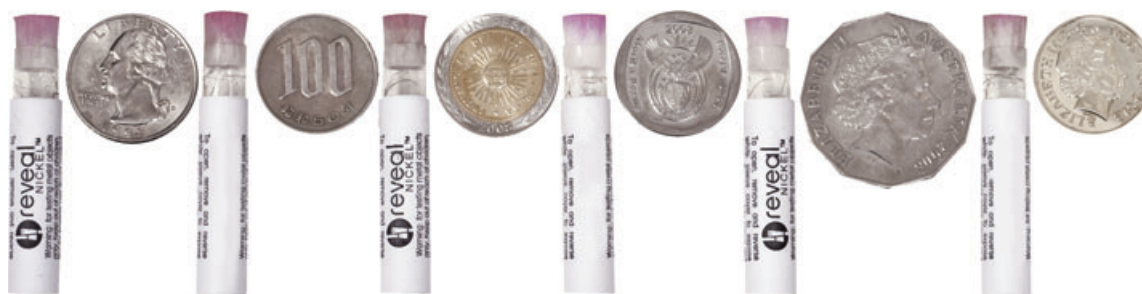
Fig. 1. Coins tested with the dimethylglyoxime test from the six major geographical regions according to the UN (4): a 0.25 US dollar coin, a 100 Japanese yen coin, a 1 Argentinian dollar coin, a 2 South African rand coin, a 0.50 Australian dollar coin, and a 0.10 UK pound sterling coin. The pink colour indicates nickel release.
