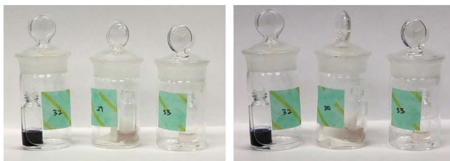
Figure 3. Chromotropic acid test for Mr. Clean Bliss gloves (samples 29 and 30) compared with positive (sample 32) and negative (sample 33) controls.
