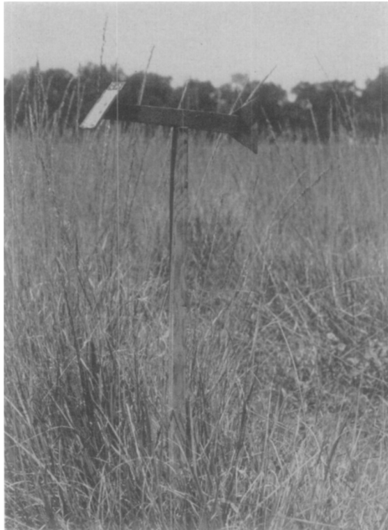
Fig. 1.—A weather vane with microscope slide holder attached, as used in this study. Grass plants in background.
