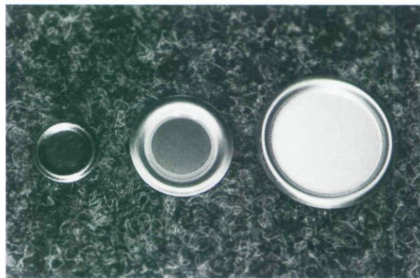
Fig. 2. Standard (left), large (middle) and extra large (right) Finn Chambers ® . Small chamber (height 0.5 mm, diameter 8 mm, maximal capacity 20 \mu l); large chamber (height 0.8 mm, diameter 12 mm, maximal capacity 70 \mu l); extra large chamber (height 1.2 mm, diameter 18 mm, maximal capacity 300 \mu l). Filter paper disks are optional. The small chamber (diameter 8 mm) is only recommended for allergy patch testing while the large and extra large chambers or similar test systems are recommended for irritancy testing.
