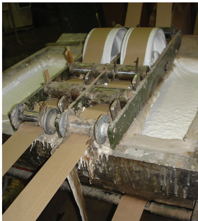
Fig. 1. Strips of brown paper being pulled through the glue tray prior to being wound on the rollers.
