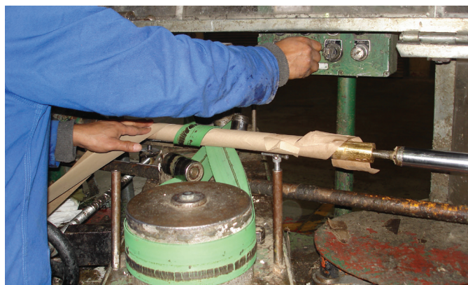
Fig. 2. The glue-coated brown paper strips being wound onto the roller to form the toilet roll cardboard core.
