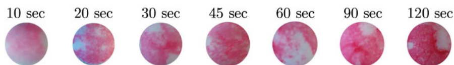
Figure 4. Color change of the ampoule tip as a function of time after testing of nickel-plated stainless steel at 3 V.
