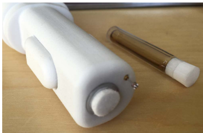
Figure 1. A photograph of the electrochemical device with an ampoule inserted and another ampoule lying next to the device.
