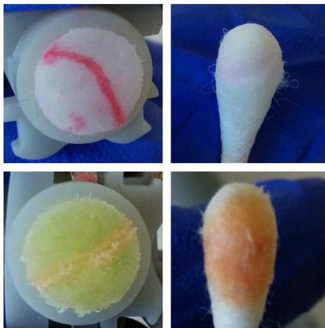
Figure 9. Comparison of an electrochemical device cotton part resulting in a positive nickel test reaction (top left) and a conventional DMG-negative test reaction (top right) when testing the same earring stick. Electrochemical device testing for cobalt showed a slight positive test reaction, which is, however, difficult to see with the naked eye (bottom left), whereas conventional cobalt spot testing clearly indicated a positive test reaction (bottom right).
