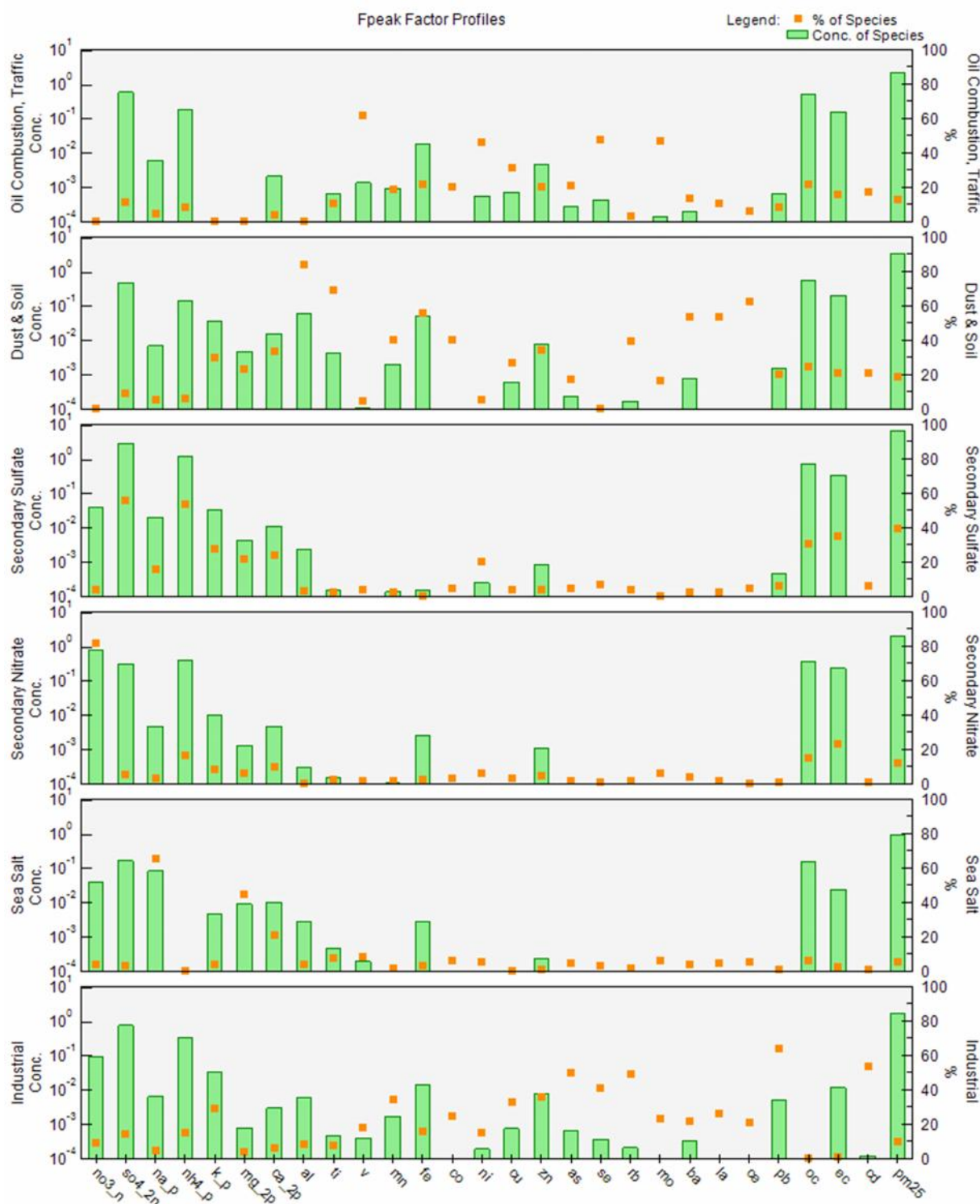
Fig. S2. Source profiles resolved from the PMF analysis for PM 2.5 in urban Nagasaki, Japan for the period March to May, 2014-2016. Left vertical axis denotes the concentration of species in µg/m 3 (bars); right vertical axis denotes the percentage distribution of chemical species across source profiles (rectangles).
