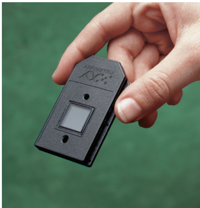
Fig. 1. A DNA microarray GeneChip. These can be used to analyse up to 47 000 transcripts (image courtesy of Affymetrix).
