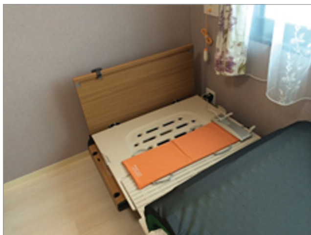
Figure 1 —Photograph showing a sheet-shaped body vibrometer set on a bed.
