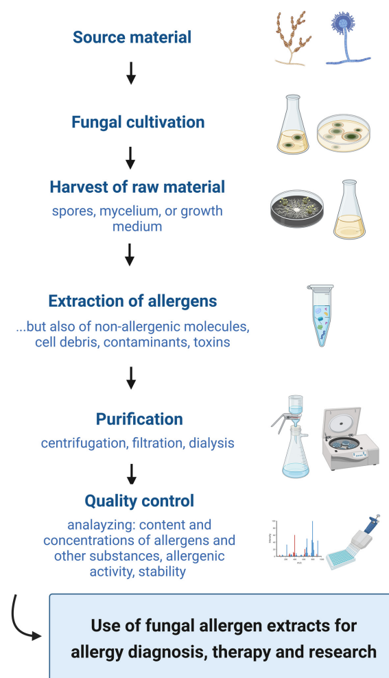
Figure 1. Production steps for the preparation of fungal allergen extracts. The manufacturing process includes the selection of the source material, the fungal cultivation, the harvest of the raw material, the extraction of allergens, the purification, and the quality control (created with BioRender.com ).
