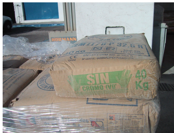
Fig. 2. A picture from 2007 taken in Lanzarote, Spain, showing a bag of cement without chromium(VI). The EU Directive restricting the marketing and use of cement containing >2 ppm chromium(VI) came into force in January 2005 (2003/53/EC).
