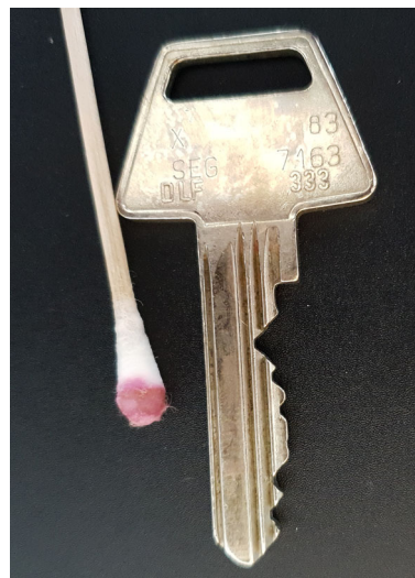
FIGURE 1 A positive dimethylglyoxime test reaction indicated by the pink colour of a cotton stick rubbed against a key
