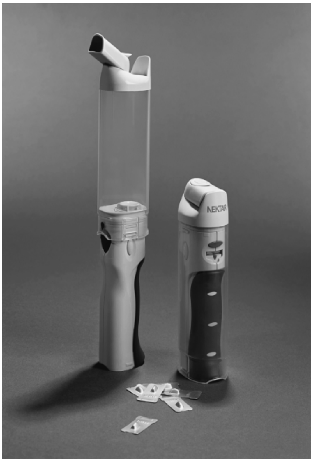
Figure 2 The Nektar Pulmonary Inhaler and Exubera™; Nektar Therapeutics Inc, Pfizer Inc and Aventis Pharma. The insulin is a fine dry powder formulation [mix of insulin (60%), mannitol, glycine, and sodium citrate]. Single-dose blisters (1 and 3 mg, equivalent to 3 and 9 units) are utilized. The air-assisted mechanism disperses the powder into a respirable cloud captured in a holding chamber 'spacer'.
