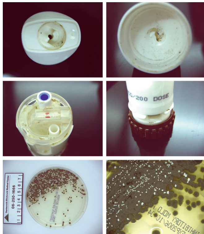
Figure 1. Mold growth is evident on multiple areas of a DPI after 12 weeks of clinical use. Growth is seen on the top and undersurface of the inhaler cap (top panels) as well as in the device interior and at the base (middle panels). Culture of the debris revealed significant growth of Candida parapsilosis and Cladosporium species (bottom panels).
