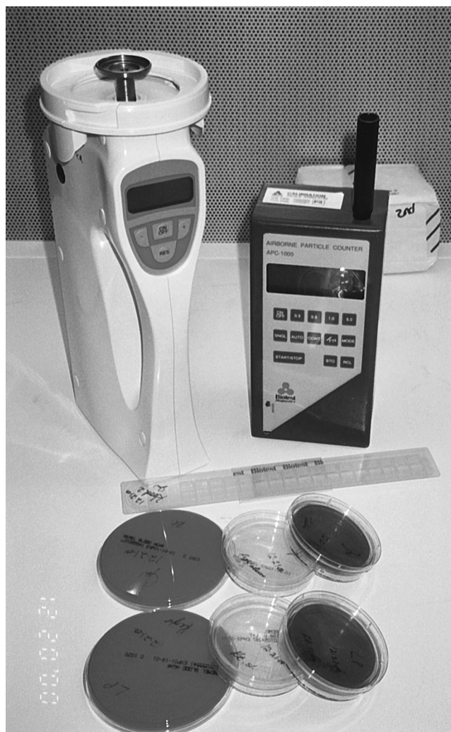
Air sampler and agar strip for viable microbes, particle counter, and microbial touch plates for surfaces, garments, and gloves.
