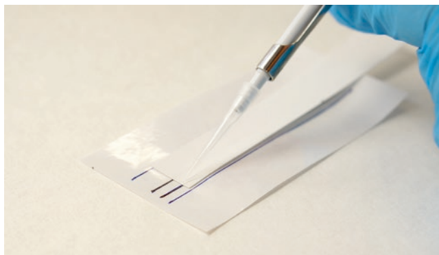
Fig. 1 Manual stripping process. Test line positioned at 0.3 cm from the membrane origin and control line at 0.6 cm from the membrane origin
