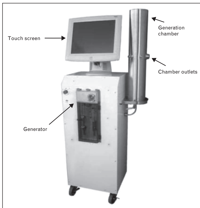
FIGURE 2. GenaSIC. An example of a close-circuit aerosol generation chamber. This figure is not original; it was previously published in [41 ■ ] (we have the permission of Dr JL Malo (corresponding author)).
