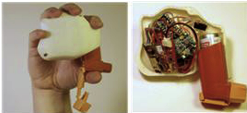
FIGURE E1. The M-ADEPT electronic medication monitor. This figure illustrates the hardware and case of the M-ADEPT electronic medication monitor. The hardware is composed of a microcontroller and a bluetooth modem. An open-source 3D modeling tool, Blender ( blender.org ), was used to design the cases housing the electronic components and the medication (constructed using a fused filament fabrication 3D printer). 3D, 3-Dimensional.
