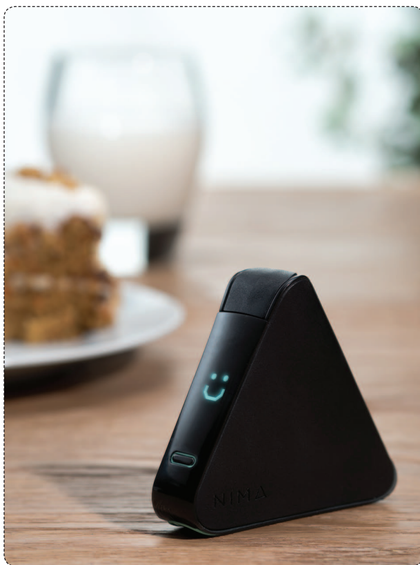
FIGURE 4 The Nima sensor consists of a mini testing kit based on developments in antibody technologies. A user can discretely insert a sample of the food to be tested into a one-time-use capsule. (Photo courtesy of Nima.)
