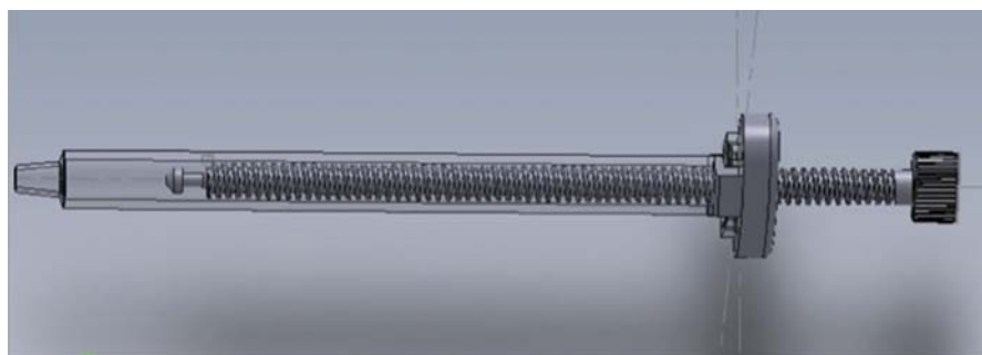
Figure 2. Horizontal view of an externally threaded plunger inside of a 1-mL syringe and an internally threaded cap that clips onto the syringe.
