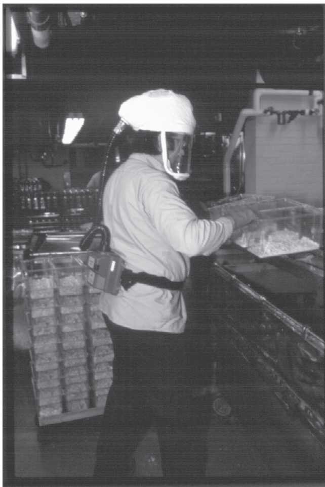
Figure 8 Worker wearing a belt-mounted powered air-purifying respirator ("PAPR") system to control aeroallergen exposure during cage cleaning operations (3M Corporation, St Paul, MN).
