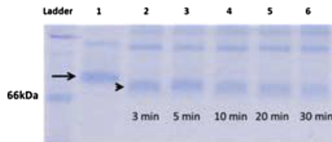
Figure 1. Native gel analysis of tissue transglutaminase and conjugate of tissue transglutaminase and toluene diisocyanate. Lane 1, tissue transglutaminase; lanes 2 to 6, conjugate of tissue transglutaminase and toluene diisocyanate produced 3, 5, 10, 20, and 30 minutes before electrophoresis. Arrow indicates tissue transglutaminase-specific band; arrowhead indicates toluene diisocyanate and tissue transglutaminase-specific band.
