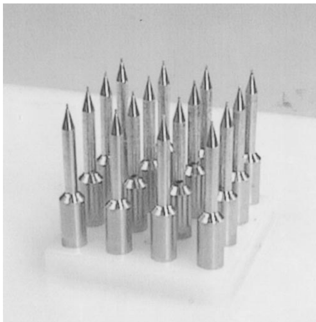
FIG. 1. Transfer stamp for protein solution transfer from 384-well microtiter plates to PVDF membranes. Sixteen individual, spring-loaded, stainless-steel pins are mounted into a POM (polyoxymethylene, polyformaldehyde, polyacetate) corpus. The pin-to-pin distance is 4.5 mm. The blunt end tip size was measured to 250 \mu\text{m} .
