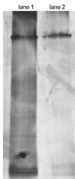
Figure 2 Nonreducing SDS-PAGE (7.5%), following silver staining to demonstrate the immunoreactive proteins during the purification of HMW Tc . Lane 1, Sephacryl 300 active fraction; lane 2, final purification step on Superose 6.
