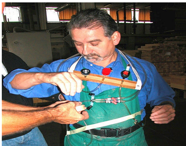
Fig. 1 Woodworker wearing the IOM sampler connected to the air sampling pump
