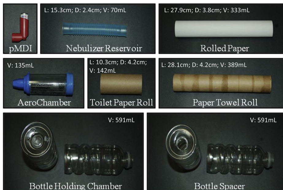
Figure 2. The accessory devices used in this study (not to scale). Pertinent dimensions of each accessory device are given: L, length; D, diameter; and V, volume. Note that the AeroChamber, nebulizer reservoir tubing, bottle-holding chamber, and bottle spacers are made from plastic. The roller paper, toilet paper roll, and paper towel roll are paper products. pMDI indicated pressurized metered-dose inhaler.
