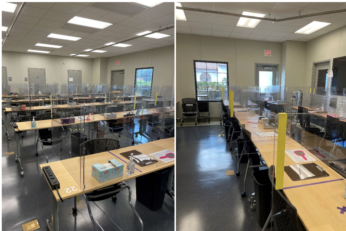
Figure. Modifications of ACC setup during the COVID-19 pandemic. Birch pollen was dispersed ( 3,500 \pm 750 grains/m 3 ) from a series of tubes along ceiling into the ACC. Two series of pollen collections and counts were done, 30 minutes apart, utilizing the Allergenco cassette system within 12 of 25 plexiglass sneeze-guard areas and in the 4 corners and center of the open chamber. Pollen counts at all sites, including inside the 12 tested sneeze-guards, were within the specified limits demonstrating good and equal antigen distribution.
