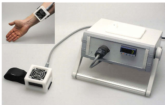
FIG 3. The TempTest 2.0/2.1 device and example of placement on the forearm for the purpose of performing cold provocation tests.
