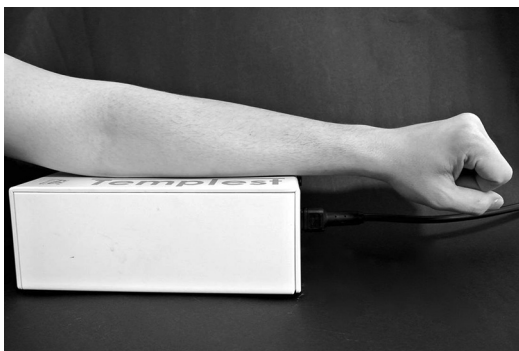
Fig. 4. Peltier element-based electronic provocation device (TempTest 4.0, Moxie GmbH) with temperatures from 4°C to 44°C to confirm cold urticaria and heat urticaria and to determine individual temperature thresholds.
