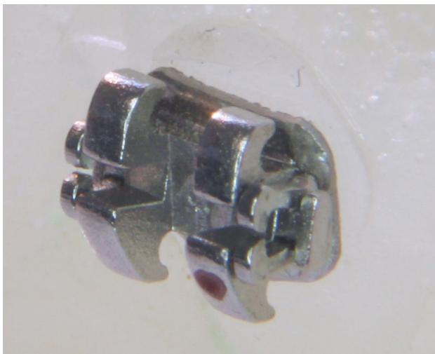
Fig. 1 Image of the self-ligating bracket system [made of stainless steel with a passive NiTi clip, 0.56 mm (0.022 in.) slot, SmartClip™, 3M Unitek, Monrovia, CA, USA] used in this study
