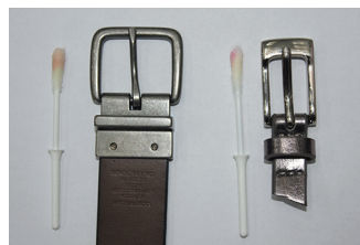
Figure 2. Examples of positive cobalt and nickel spot test reactions indicating cobalt and nickel release in sufficient amount to elicit allergic dermatitis in sensitized individuals. Left, (Cobalt) A positive reaction as indicated by an orange-red coloration of the yellow cotton stick. Right, (Nickel): A positive reaction as indicated by pink coloration of a white cotton stick.
