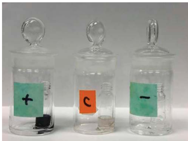
Figure 2. The Co-Flex NL bandage (c) shows a mild purple discoloration compared with positive (+) and negative (–) controls, indicating formaldehyde release.
