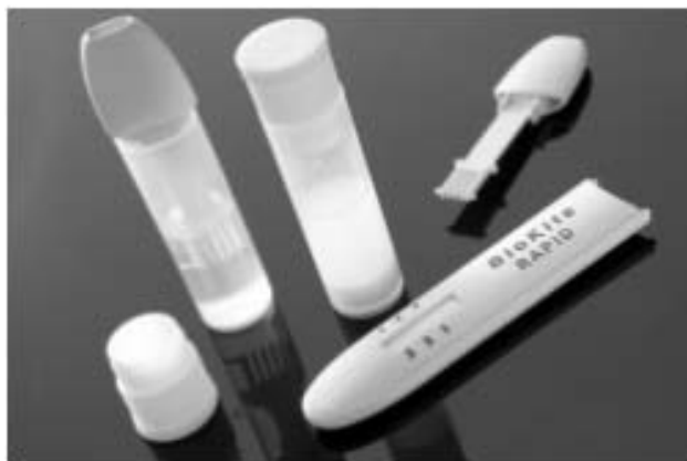
Figure 1. Rapid lateral flow-type test components; sample application comb at top right; test device at bottom right.
