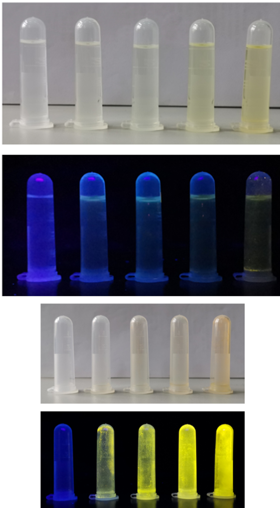
Fig. 7. (a) The colors of the mixed solution containing 0.5 wt% salicylaldehyde and different concentrations of PPD under visible light (top) and 365 nm UV light (bottom). The PPD concentrations were: 0, 250, 500, 1000, 10,000 \mu\text{g L}^{-1} (b) The colors of the residue in the plastic tubes under visible light (top) and 365 nm UV light (bottom). (For interpretation of the references to color in this figure legend, the reader is referred to the Web version of this article.)
