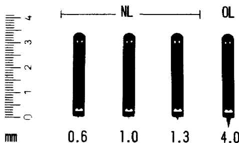
Fig. 1. Three of the new lancets (NL) with point lengths 0.6, 1.0, 1.3 mm and, on the right, the old lancet (OL).
