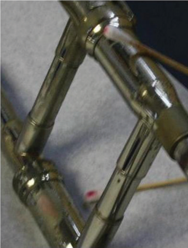
Figure 3. Dimethylglyoxime-ammonia testing (+) at points of plating wear on the instrument.
